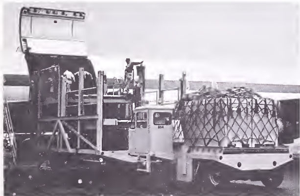
FIGURE 1.—Strawberries assembled on a master pallet covered by a cargo net being loaded aboard airfreighter.
